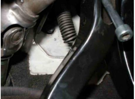
Note: image shows spring attached to clutch pedal.
