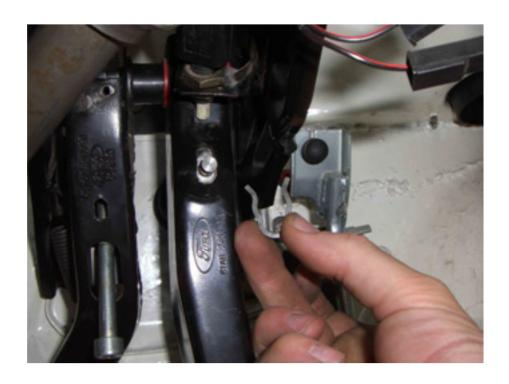
**4).** Slide the shaft out keeping note of where the washers and spacer bushes came from, and remove the brake and clutch pedals. (Note: the shaft will only slide out one way and that is towards the centre of the car)
