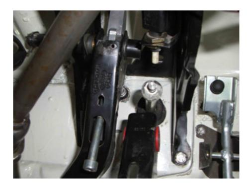
**5).** Remove the spring from the original clutch pedal ratchet system. Then hook the larger eyed end of the spring onto the pedal box at the position shown in Image below.
