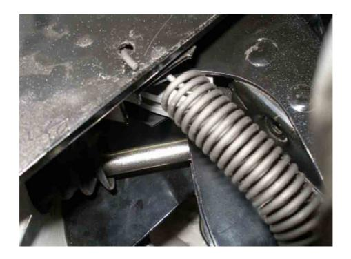
Note: This image shows the existing hole in the left hand side of pedal box.
