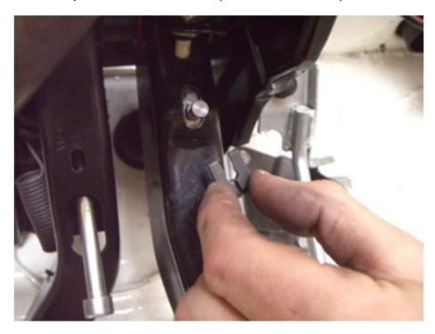
**3).** Remove the clip on the shaft on the right hand side of the brake pedal in between the pedal box and the pedal.
