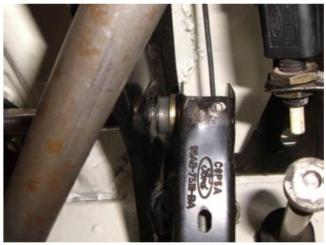
**8).** Slide the quadrant in between the bushes at the top of the clutch arm, making sure the nipple retention part of the quadrant is at the top.
